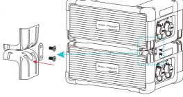
3: Install the protective corners in the following order: first, align the side with the positioning structure then snap the front side into place. Install them one by one until they are properly
