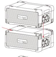
2: Use screws and metal connecting piece to secure the stacked power packs from top to bottom.
