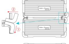
4: After installation, as shown in the diagram, to ensure safety, stack a maximum of four EP3000-48V power packs. (The protective corners in the middle of the power packs are for aesthetic purposes only and do not provide structural strength.)
